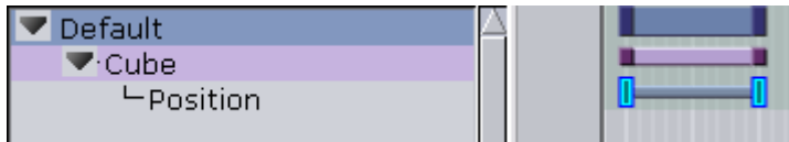
Figure 89: Example of cube with animated position; two keyframes and bar between
