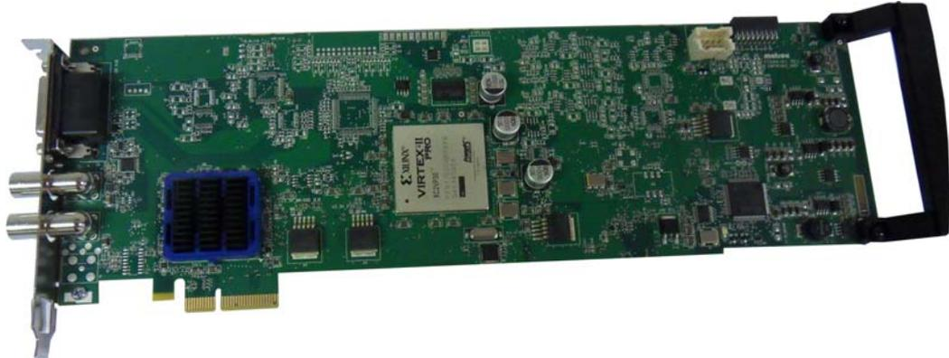
Matrox DSX LE2/CG is HD ready, has 2 video outputs, but no video input. It is used for outputting fill and key signals, and is a useful card in systems that do not need live video input or codec support.
