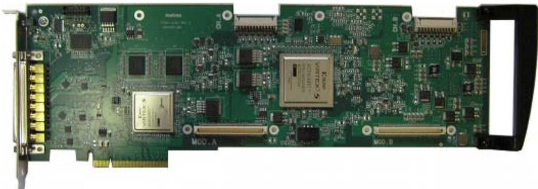
The Matrox X.mio cards are used as Vizrt's **HD** and **SD** multi-channel video- and audio **I/O** solution, replacing the Pinnacle Targa 3200.
