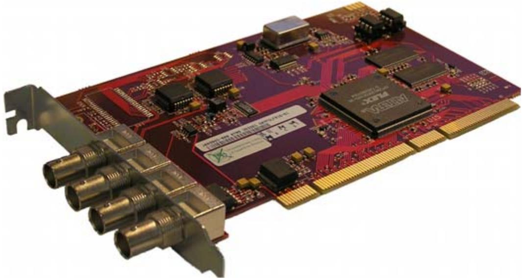
BlueFish444 Iridium|SD is the native successor of the [Digital Voodoo DeepBlue LT](#) and the predecessor of [BlueFish444 SD Lite Pro Express](#), providing Fill, Key, [GenLock](#) and Composite Fill connectors. The Iridium|SD is fully compatible with older DeepBlue-LT installations.
