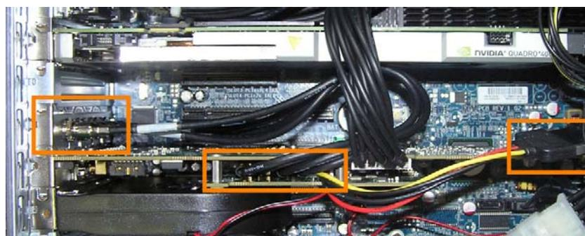
6. Mount the slot panel with the 4 additional inputs in any free slot and connect the power for the X.RIO. Also, make sure the cables do not touch any fans
