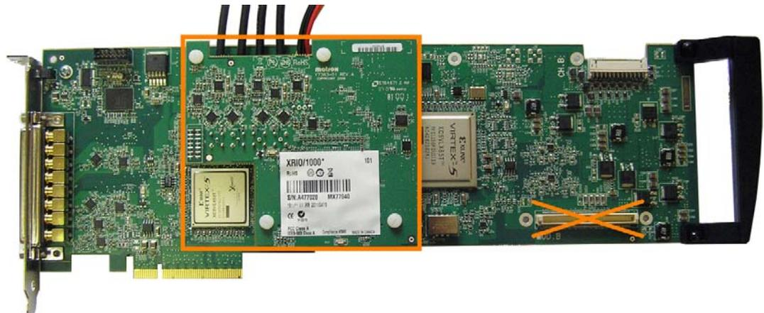
3. Mount the X.RIO on the XMio2 card "Mod A" connector. The Mod B connector will not work
