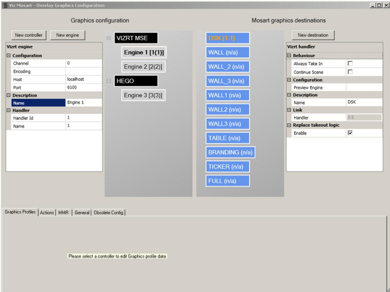
On the left hand side are the Engines and Controllers, while on the right hand side are the Destinations. The Overlay Graphics Configuration - Property Tabs are available at the bottom of the window.
