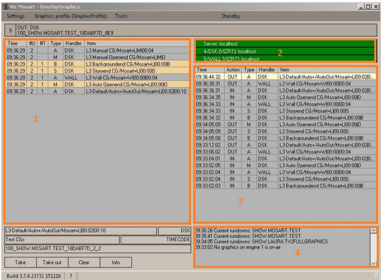
The Overlay Graphics user interface consists of four main areas (referenced as [1] to [4] in the text) as well as a top main menu, graphic status line under the main menu and an info line at the bottom of the main window.
