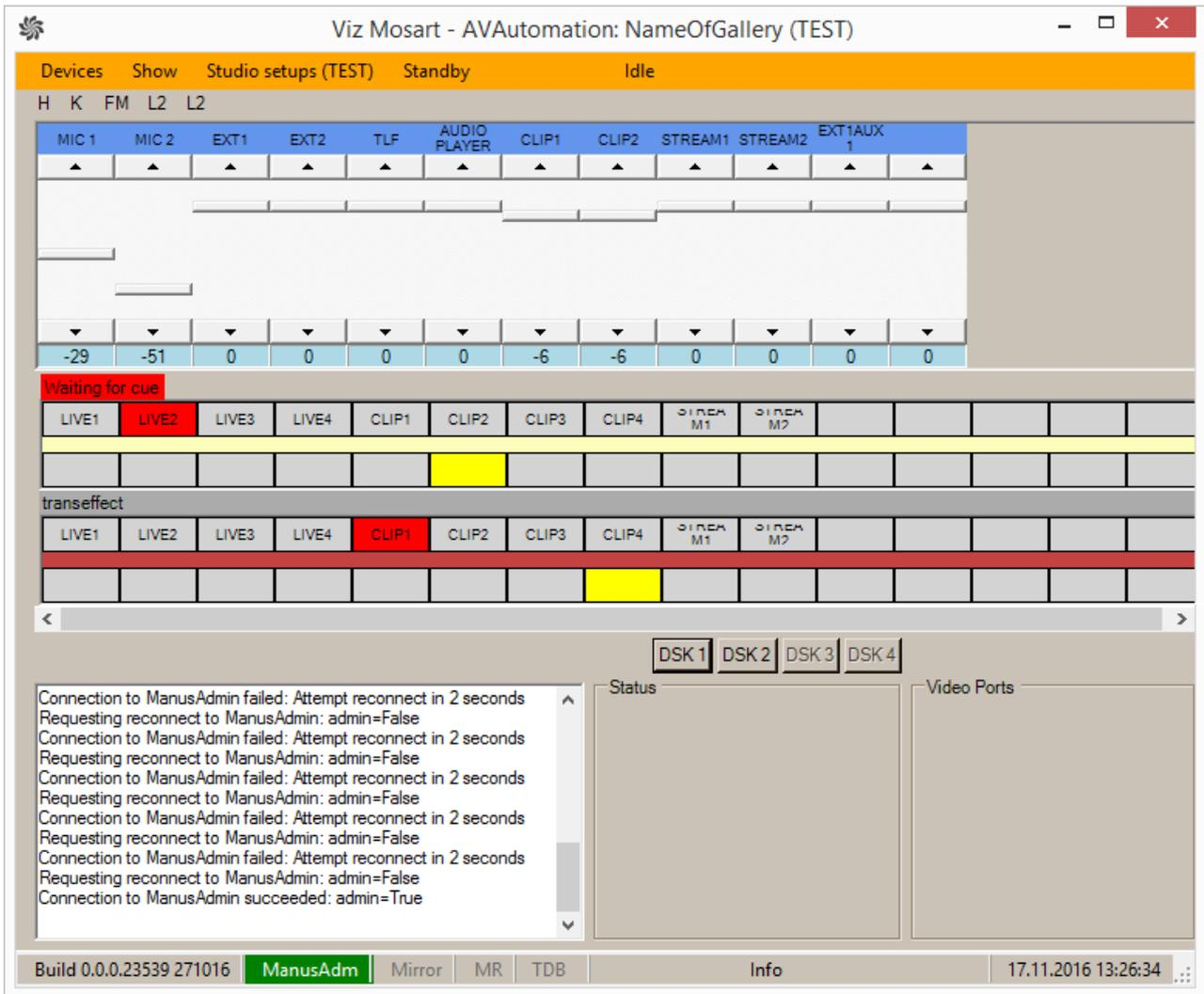
AV Automation (MMAVAutomation) is where all Viz Mosart connected broadcast devices (except Overlay Graphics engines) are controlled. Full-screen graphics is also controlled here.
