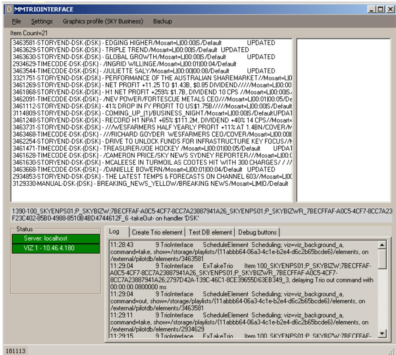
Trio Interface is for controlling and monitoring overlay graphics for Viz Engines. It can be used with either Viz Trio or Viz Pilot, and requires the use of the Media Sequencer to issue commands to the Viz Engine.
