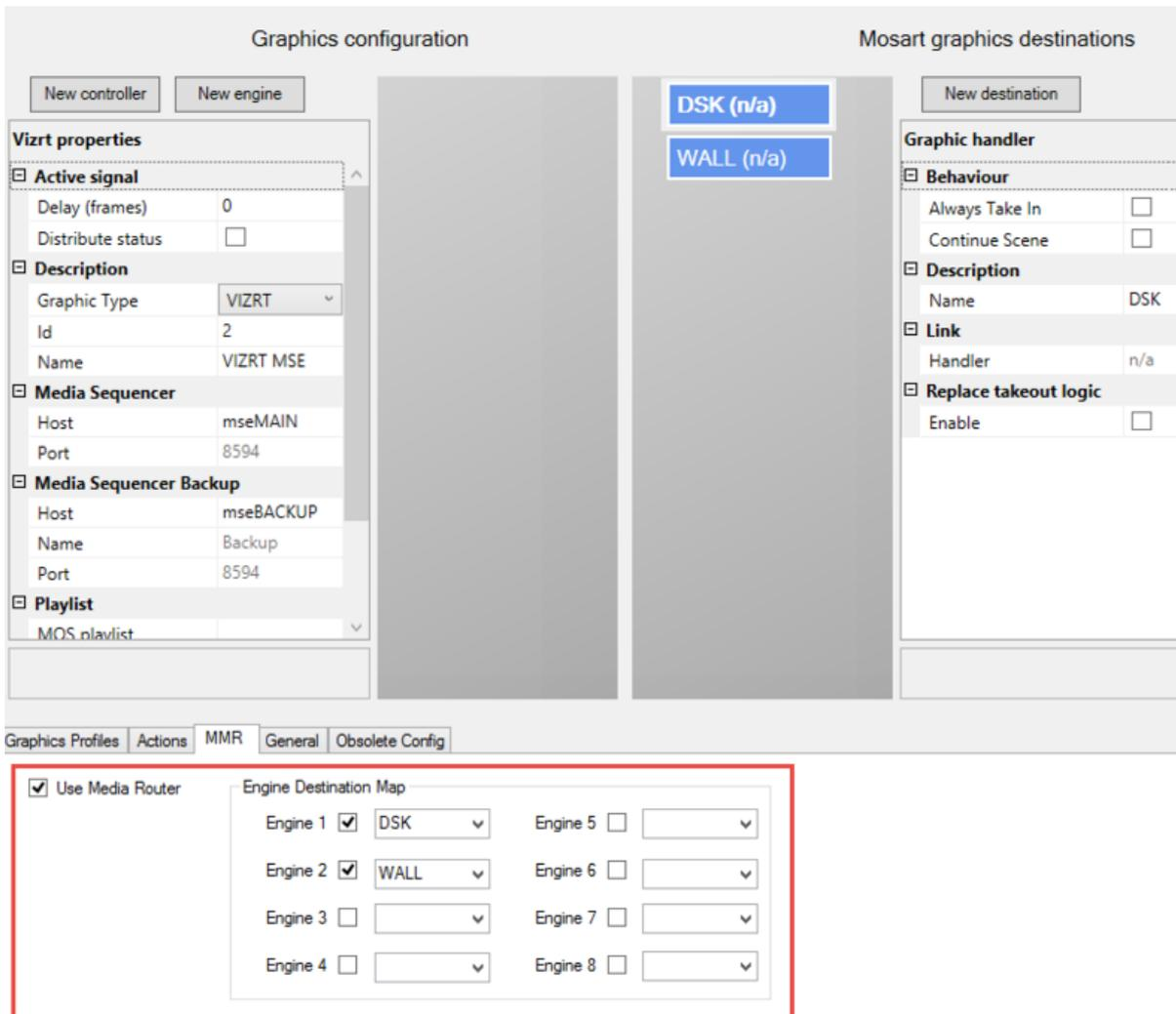
**Note:** When using Media Router for OverlayGraphics, it is not necessary to create any Graphics configuration (left side). However it is required to specify all graphics destinations (right side) together with an optional mapping between engine number and graphics destination.
