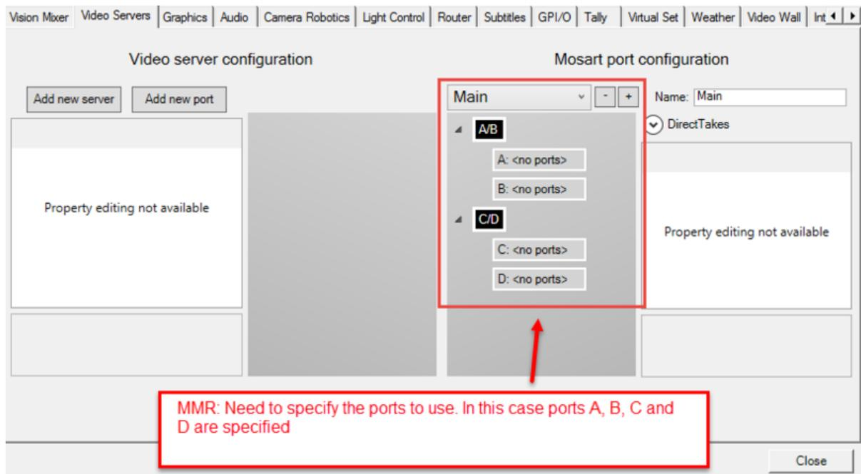
**⚠ Note:** In the example above, it is only necessary to specify the Mosart port configuration (right side). The static video server configuration (left side) may be left empty.
