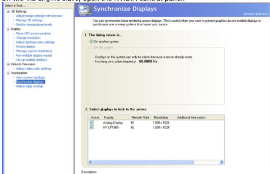
1. On the Viz Engine slave, open the NVIDIA control panel.
