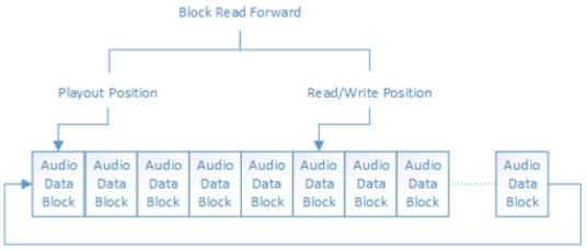
All sound devices use a ringbuffer that stores data until it is sent out to the audio channels, and this ringbuffer is organized in blocks of data. All sound hardware defines a distance in blocks (or bytes) that needs to be maintained. For almost all devices on the market a distance of six blocks is sufficient to have a clean output without artifacts.
