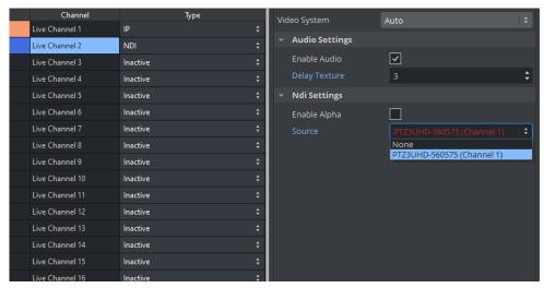
If at least one NDI input is configured during startup, Viz Engine scans the network for NDI senders. All discovered sources are shown in the drop down menu.
