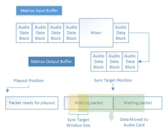
After mixing the packages received from the Matrox board, the blocks of audio data are moved to the Matrox output buffer. This buffer is organized as a ringbuffer and holds one second of data and this is the maximum delay that can be achieved with the described mechanism.
