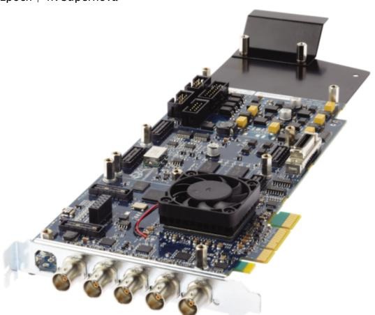
The Epoch | Supernova is a full-length PCIe card with five bi-directional multi-format I/O BNC connectors that support a number of configurations with up to two dual link channels or four single link channels. For use with Viz Engine, the card needs to be configured with two inputs and two outputs.
