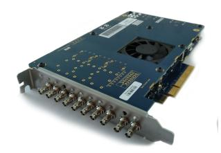
The Kronos K8 is a full-length PCIe card with ten HDBNC connectors. Eight of those are used for SDI IO, the other two are reference connectors. For use with Viz Engine, the card needs to be configured with four inputs and four outputs. The connectors support SD, HD 1.5G, 3G, ASI, AES and LTC as either input or output. In addition the card has a reference input and a reference output connector.
