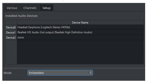
The audio system is able to use any installed DirectSound capable audio device. On every device, up to 16 channels can be used.
