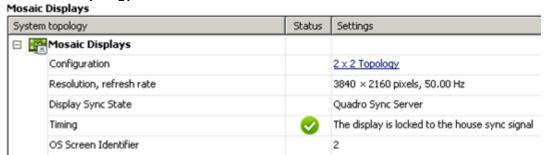
The View System Topology panel reports that The display is locked to the house sync signal for one of the connected displays. For the other connected displays, the report states that The display is locked to the frame lock sync pulse.
