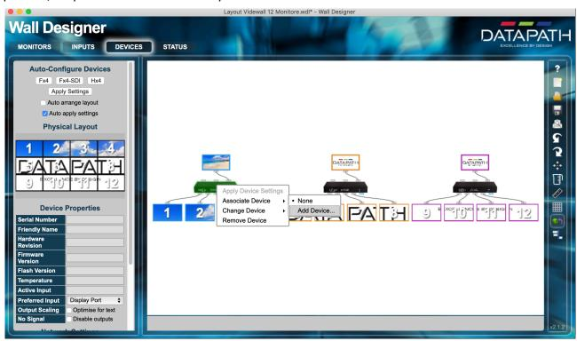
Right click on the **Datapath** and assign the correct one. If it is missing from the list, please manually add the IP number of your device. (This can be obtained by connecting it via USB). Once you click on the **Apply Settings** button, the configuration activates and the nVidia should recognize three virtual monitors with a resolution of 7680x1080 each. Verify the input by clicking on the input image(s). Once this step has been completed, you can continue by creating your nVidia mosaic:
