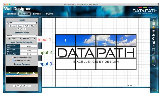
Press **Adjust Capture Regions** if you need to adjust the area the input captured by the various monitors. The alignment of monitors can be fine tuned pixel accurate. Any bezel correction needs also be done here. Make sure the displays align correctly to the configured input.
