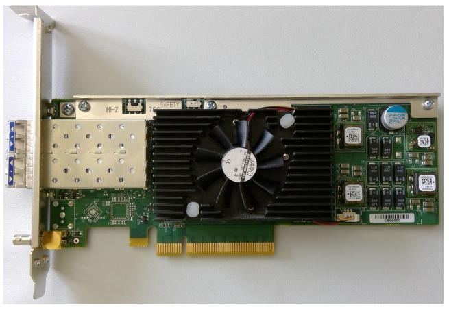
The card contains two enhanced small form-factor pluggable (SFP+) slots, or "bays". In the lower bay is **SFP A**, and hosts input and output channels 1 through 4. The upper bay houses **SFP B**, which hosts all of the redundant channels used with SMPTE ST 2022-7. The board does not have any SDI inputs or outputs. There is one Mini-BNC connector used to connect the card to the house genlock signal. However, the card can also be locked to a SMPTE ST 2059 conform time signal, sent via the SFPs.
