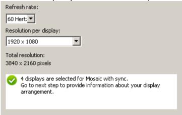
2. Once Mosaic is configured and the G-Sync device has been locked to the house-sync, the topology in the NVIDIA control panel should look as follows, with the report for one of the connected displays stating **The display is locked to the house sync signal**.
