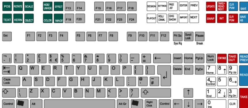
The keyboard contains two rows with extra function keys which have been assigned to different Viz Trio actions. The keyboard has its own configuration software. A Viz Trio configuration file must be loaded to create the correct keyboard map. In the Viz Trio client a keyboard mapping file must be imported to assign the correct actions to the keys. This is pre-installed on all Viz Trio clients, so normally these settings will not have to be changed.
