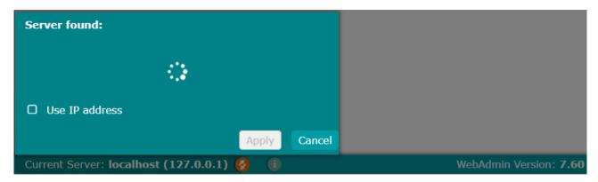
After scanning the network for available servers, the options are displayed, showing the hostname and IP address. By clicking on the server and if the access is enabled, the page is forwarded to the CodeMeter WebAdmin of the server.
